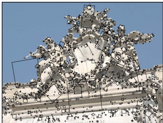
Fig. 4. Example set of detected SIFT features. Each detected SIFT feature is displayed as a black box centered on the detected feature location. SIFT detects a canonical scale and orientation for each feature, depicted by scaling and rotating each box.
