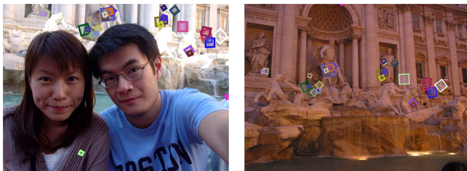
Fig. 5. SIFT feature matches between two images of the Trevi Fountain. Each match is shown by a small square of the same color in both images. Matches are found despite the fact that the images are taken at different times of day, and in one image the scene is significantly hidden by people in the foreground.
