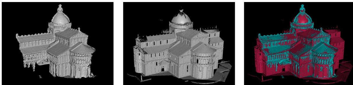
Fig. 13. Comparison of a reconstructed geometry model with ground truth. Left: merged model of the Duomo in Pisa reconstructed from a community photo collection with 56 images. Middle: laser scanned model of the Duomo serving as ground truth. Right: false color rendering of the two registered models overlaid on top of each other demonstrating that the two models match closely. (Scanned Duomo model courtesy of Visual Computing Group, CNR, Pisa, Italy.)
