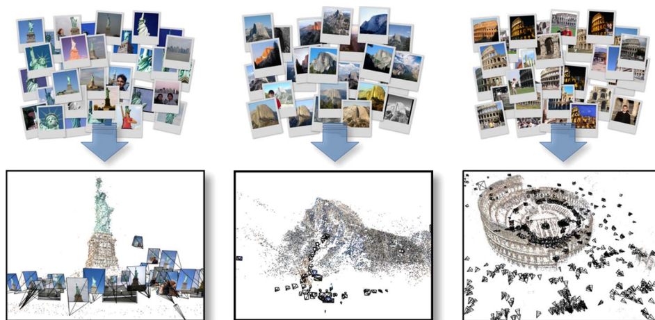
Fig. 2. 3-D reconstructions from Internet photo collections. We take image results from keyword search (top), and automatically recover camera positions and scene geometry (bottom).
