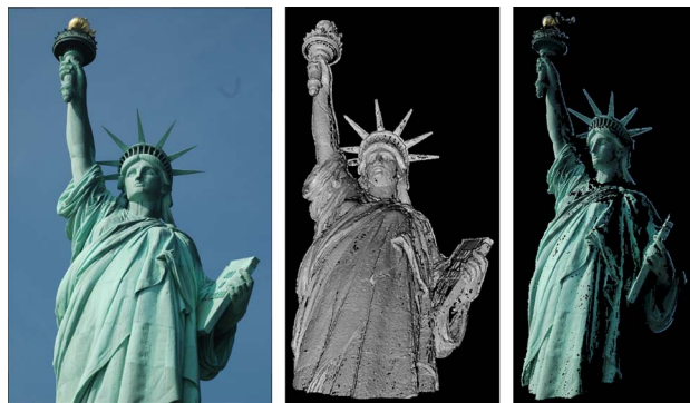
Fig. 12. A view of the Statue of Liberty and the corresponding depth map. Left: original input image from a community photo collection. Center: reconstructed depth map rendered from the original camera viewpoint. Right: the same depth map textured with the input image and rendered from a novel viewpoint.
