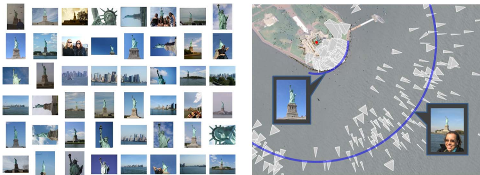
Fig. 19. Paths through the Statue of Liberty photo collection. Left: several Flickr images of the Statue of Liberty, from a collection of 388 input photos. Right: reconstructed camera viewpoints for this collection, revealing two clear orbits, shown here superimposed on a satellite view. Our goal is to automatically discover such orbits and other paths through view space to create scene-specific controls for browsing photo collections.
